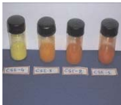
Quantum dots changing colour with reducing particle size
